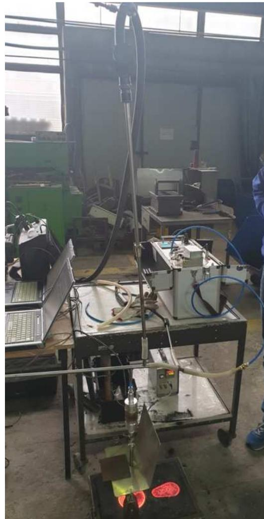
Figure 4. Test station for measurement of BTEX and PAHs content in released gases
