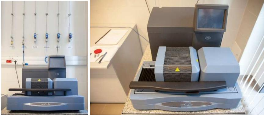
**Method:** TG/DTG//DSC method, temperature range 30-900 °C, heating rate 10 °C/min, inetr atmosphere (25 ml/min), corundum or graphite crucibles or with a hole in the lid (85 µl).
