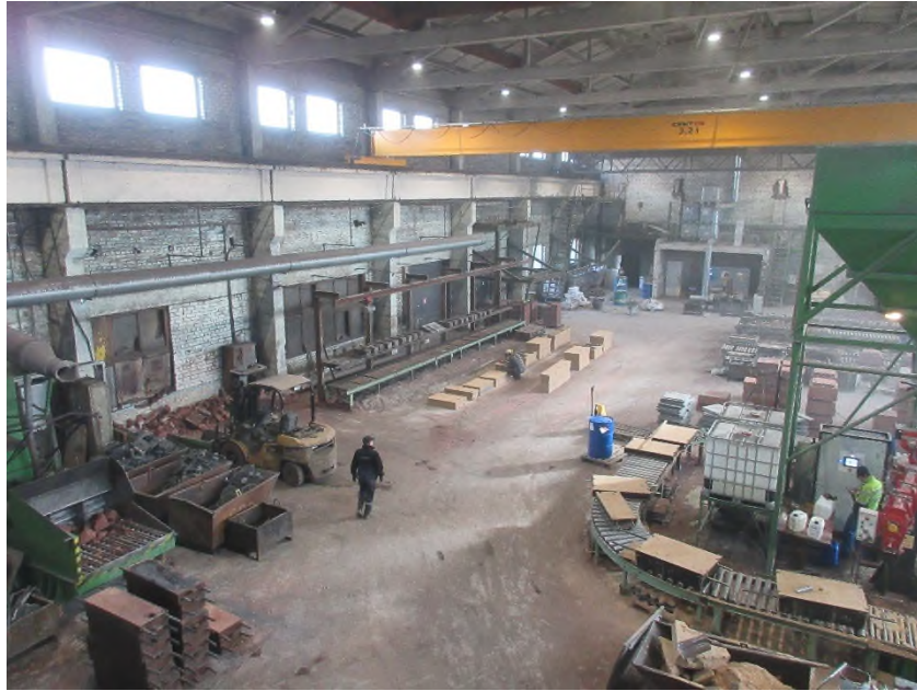
Figure 1. Overview of the foundry. At the back is the induction furnace and on the right the sand mixer.
