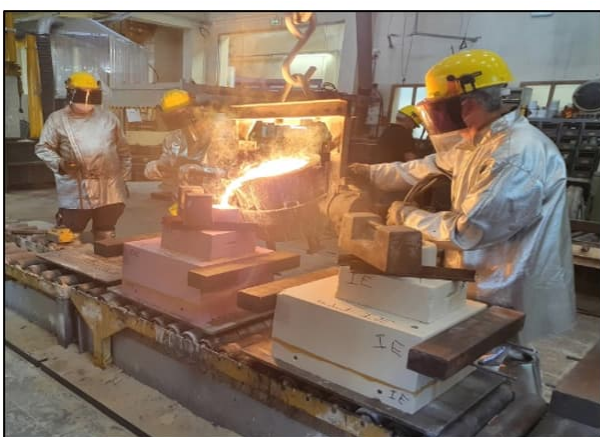
Steel GS240 pouring (30 kg/mould – casting weight = 12 kg)
