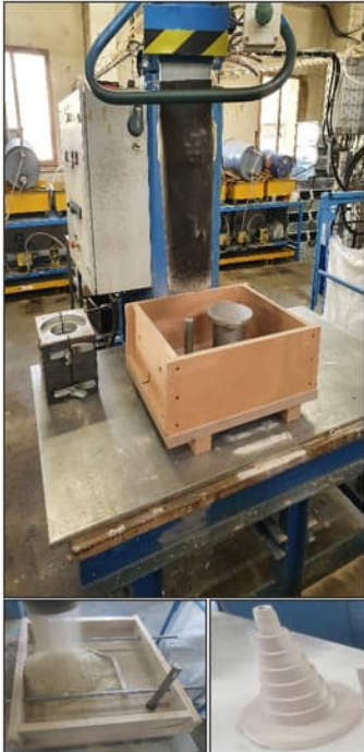
Moulds and cores making pouring
