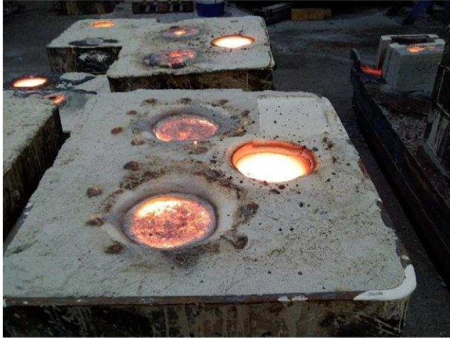
Photo 43. No fumes from an inorganic mould
