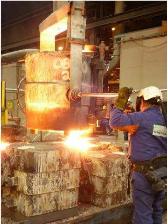
Photo 17. Pouring of melted metal into the inorganic test moulds.
