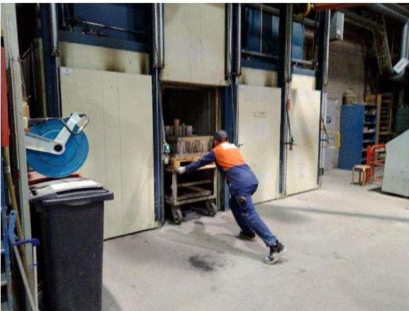
Photo 14. Core heating furnace.
