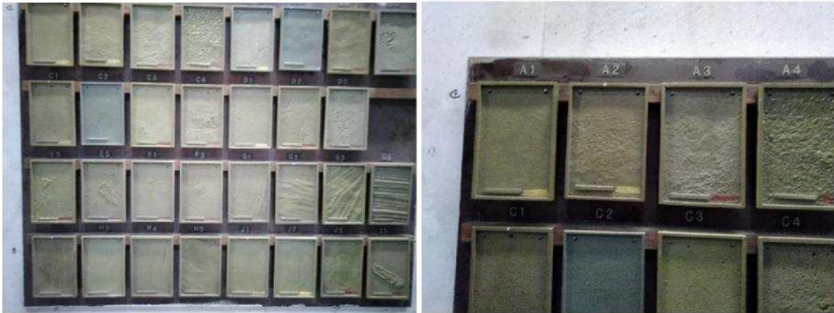
Photo 26. Reference surface quality models at Karhula Foundry
