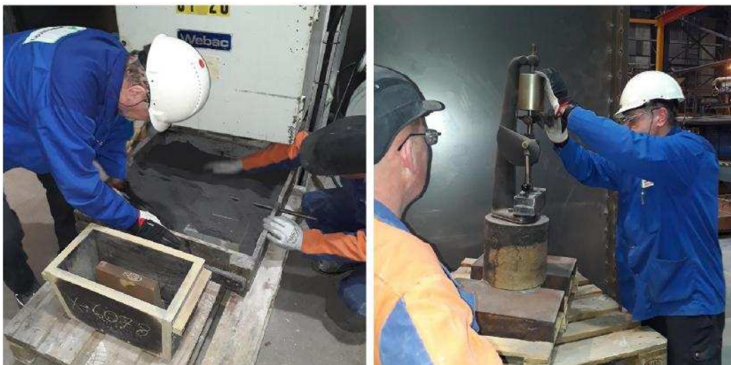
Photo 1. Laboratory mixer, hand moulding and making of sand test bars.
