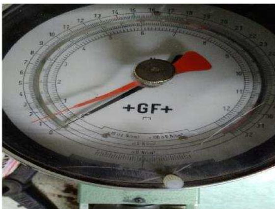
Photo 41. The result of sand bar bending test after 24 h.
