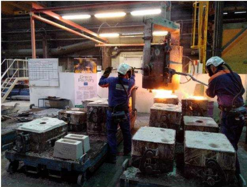
Photo 23. Pouring from a ladle
