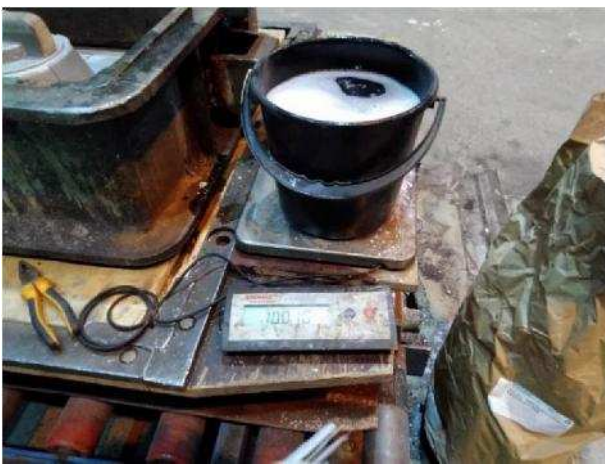
Photo 12. Measuring of binder weight
