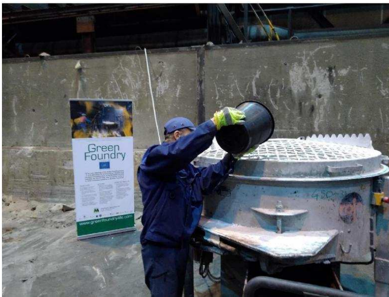
Photo 30. Test mixer, adding of binder during mixing
