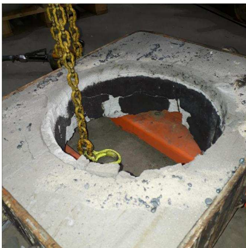
Photo 8. Chamber test mould after cooling. Black burned sand around the casting.
