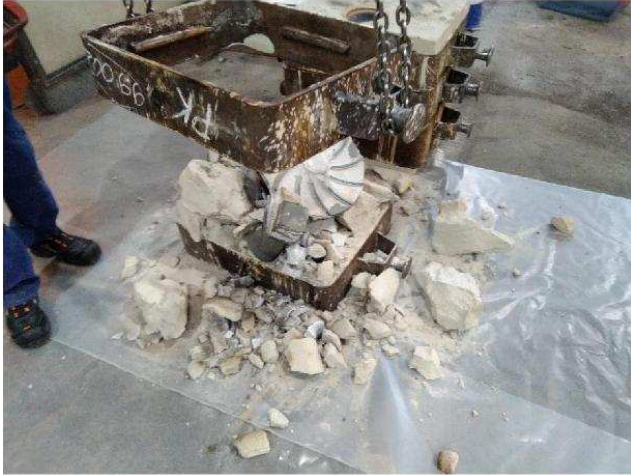
Photo 25. Manual opening of moulds
