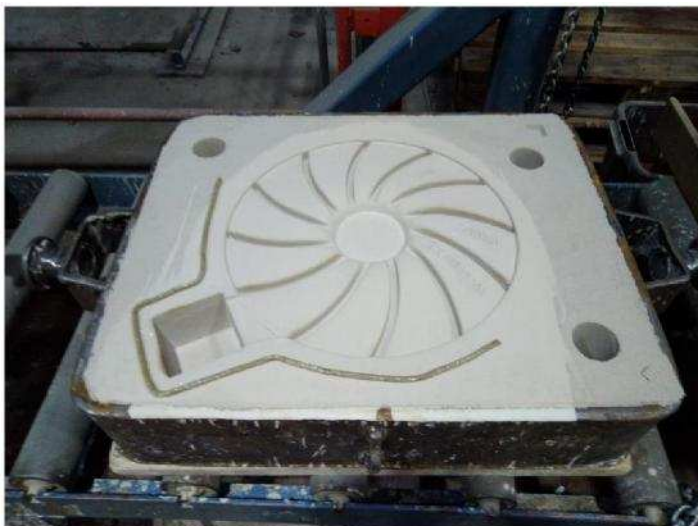
Photo 22. An example of coated mould.
