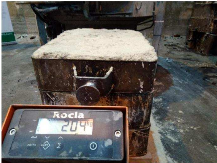
Photo 33. The amount of sand in the test mould
