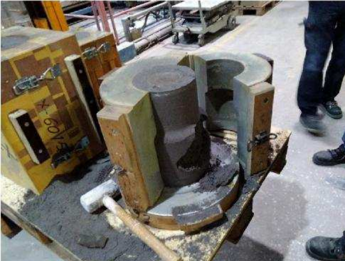
Photo 15. Braking of a core due to a lack of proper drying
