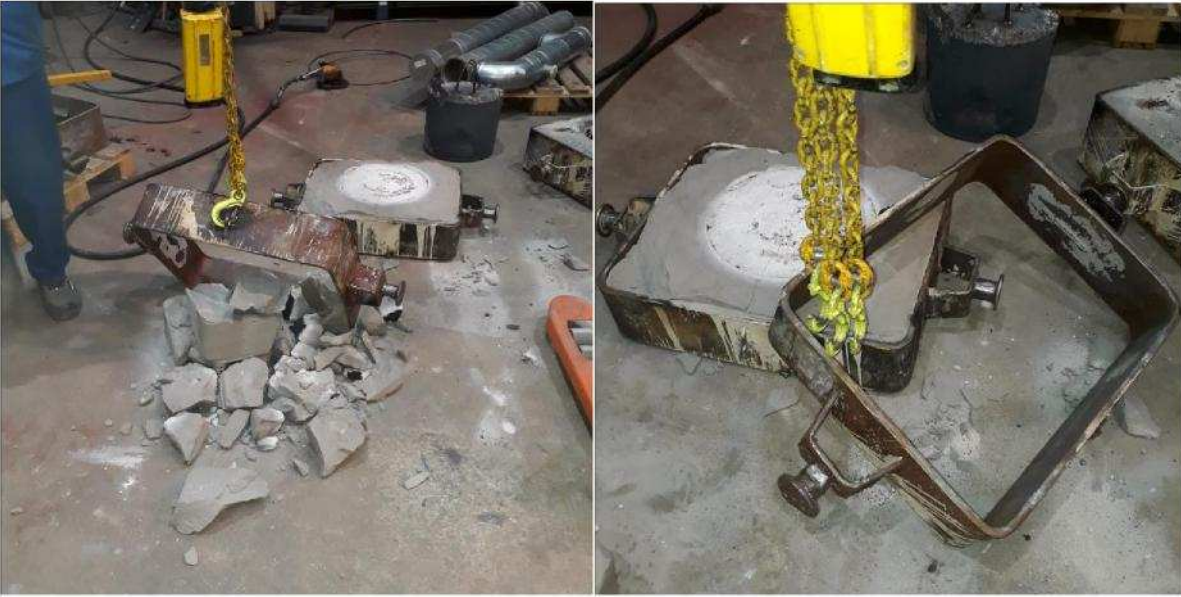
Photo 9. Breaking of the chamber test mould.
