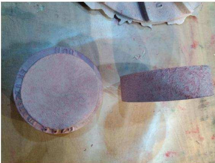
Photo 29. Dye penetrant inspected test castings. No cracks or gas porosity holes existed.
