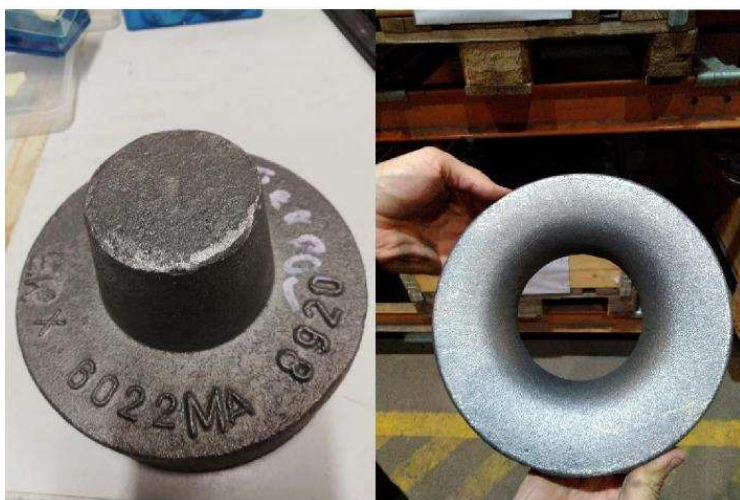
Photo 46. Surface qualities of castings made by inorganic binder nr.3 (left) and Alphasert (right).
