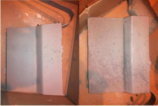
Photo 19. Test cast from coated mould, left, and from uncoated mould, right.
