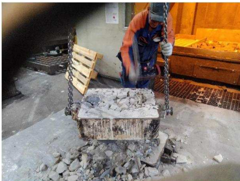
Photo 45. Manual crushing of moulds
