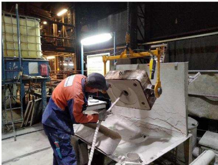
Photo 42. Coating of the test moulds
