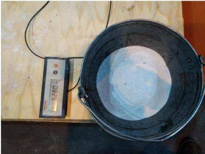
Photo 37. The amount of loose sand
