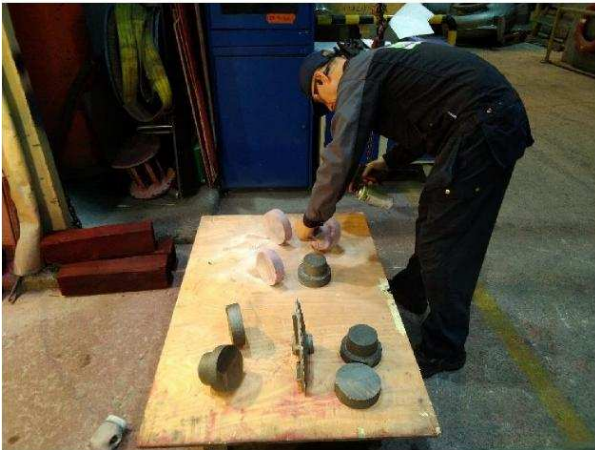
Photo 28. Dye penetrant inspection (DPI)
