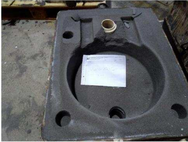
Photo 17. Cracks in the test mould due the high strength.
