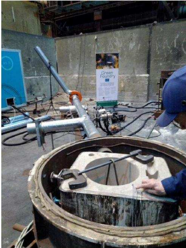
Photo 34. Test mould inside the chamber. The locations of the thermoelements.
