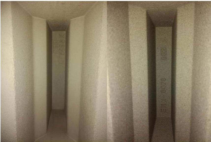
Photo 18. Coated mould, left and uncoated mould, right.
