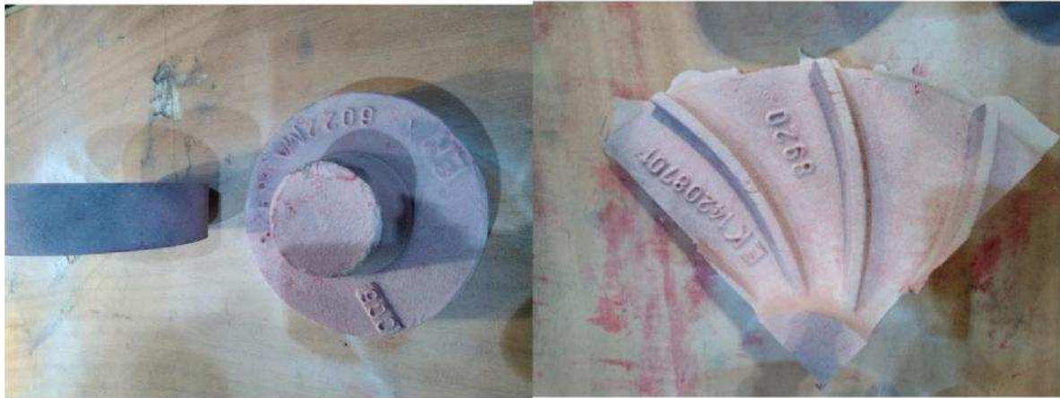
Photo 47. Dye penetrant inspected test castings. No cracks or gas porosity holes.
