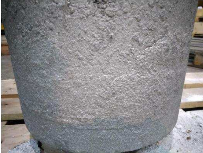
Photo 38. Surface quality of the chamber test casting (after sand blasting), no coating was applied.
