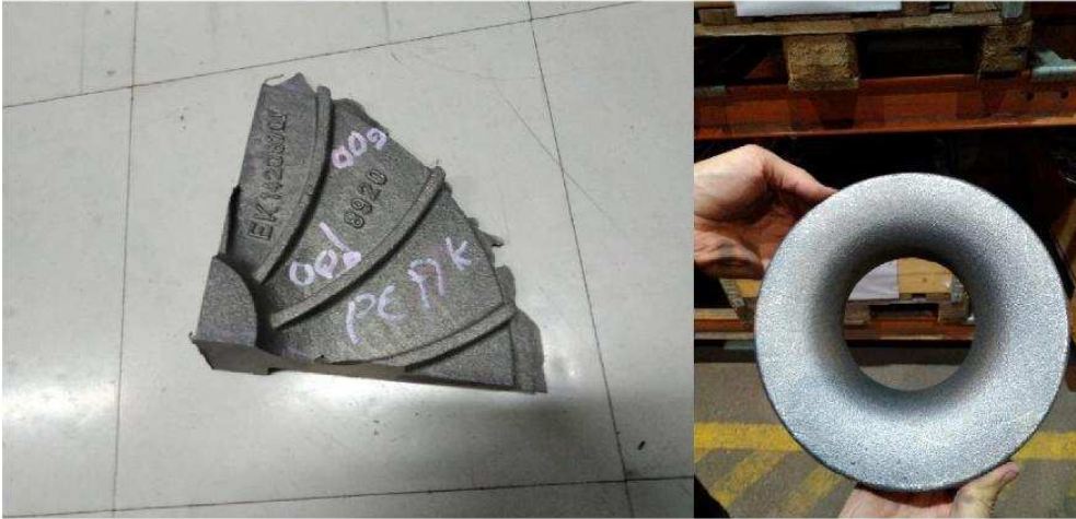
Photo 27. Surface qualities of castings made by using inorganic binder nr.2 (left) and Alphaset (right)
