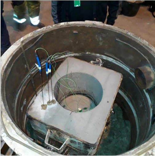
Photo 5. Test mould in the chamber, thermocouples installed.
