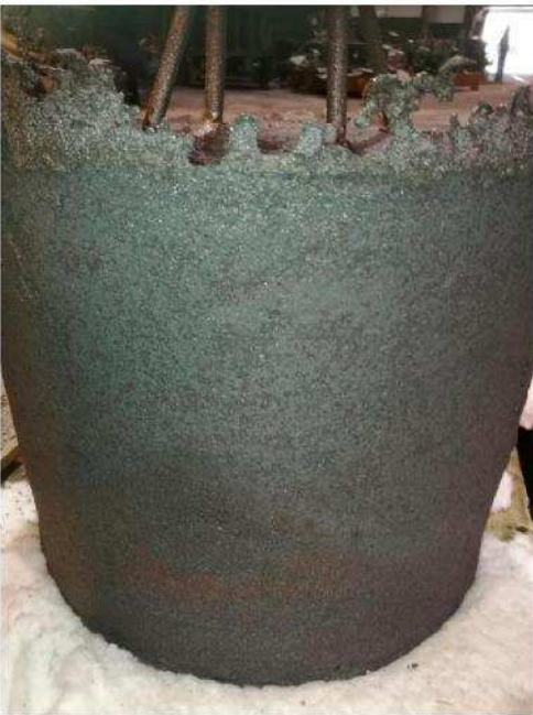
Photo 10. Surface quality of the chamber test cast.
