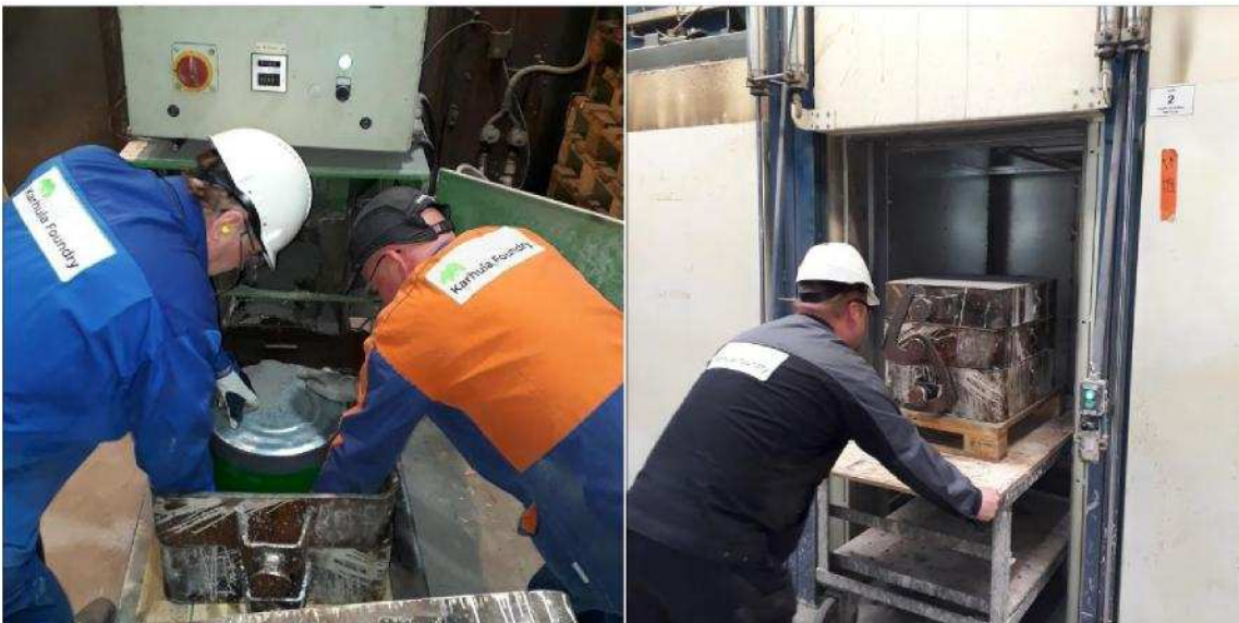
Photo 4. Hand moulding and heating oven. Temperature 160C°, drying time four hours.
