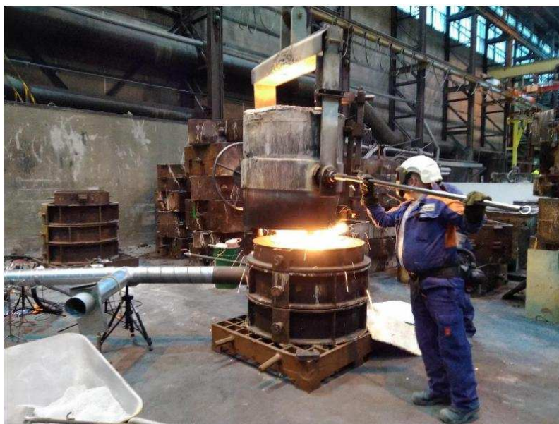
Photo 35. Pouring into the chamber test mould
