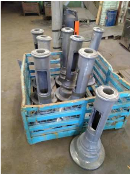
Figure 18. Test casting made by Geopol binder system.
