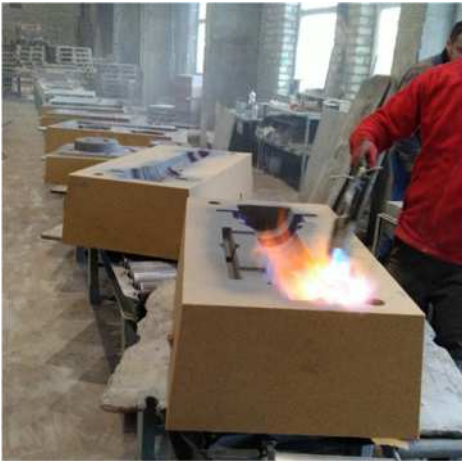
Figure 15. Drying of the coating with flame burning.
