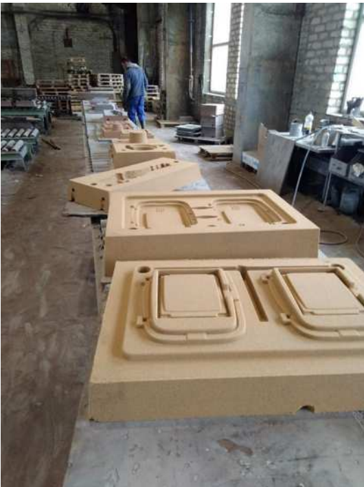
Figure 7. Examples of the moulds made by Peak's binder system
