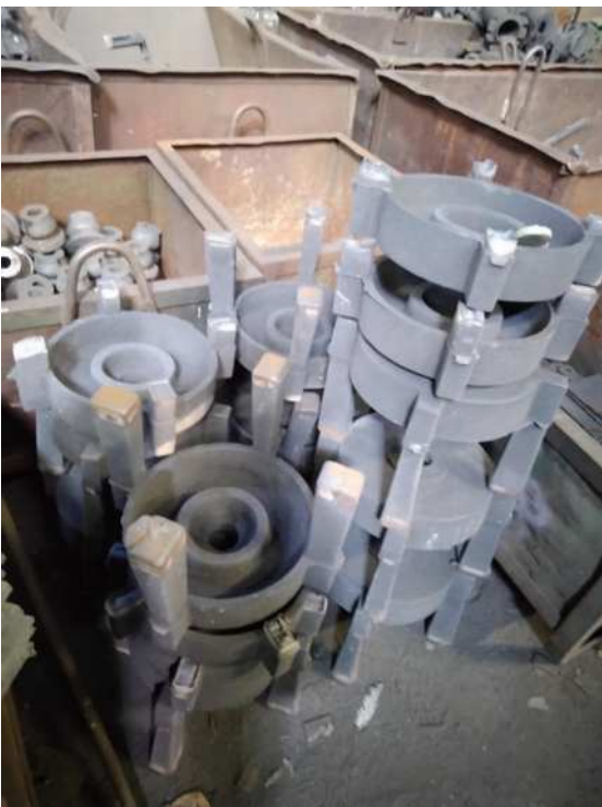
Figure 12. Test castings made by Peak's binder system after shot blasting.
