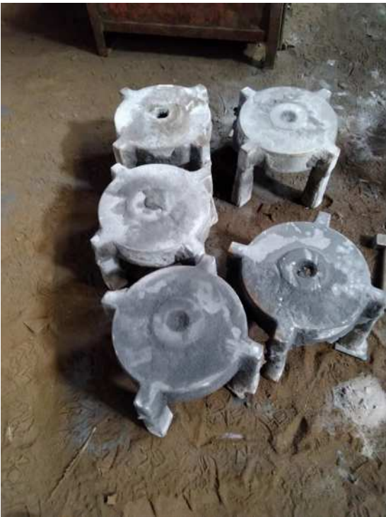
Figure 11. Test castings made by Peak's binder system before shot blasting.
