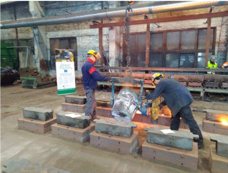
Figure 9. Test cast of the moulds made by Peak's binder system.
