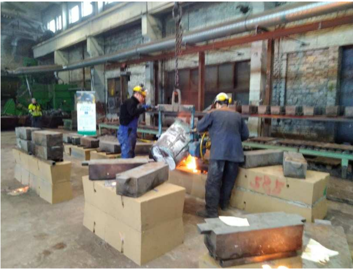
Figure 16. Test cast of Geopol moulds. Small leakage in one mould, left.
