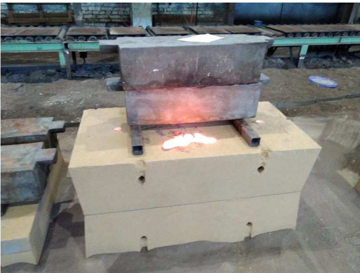
Figure 17. Geopol test mould. No visible fumes were emitted. Photo was taken 5 minutes after pouring.
