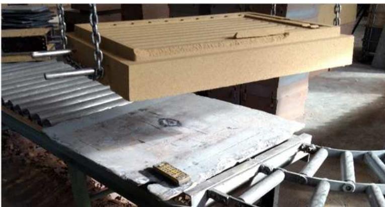
Figure 13. Mould made by Geopol, broken during stripping.
