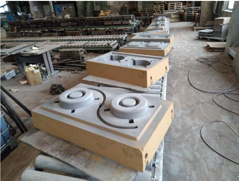
Figure 8. Coated moulds made by Peak's binder systems.
