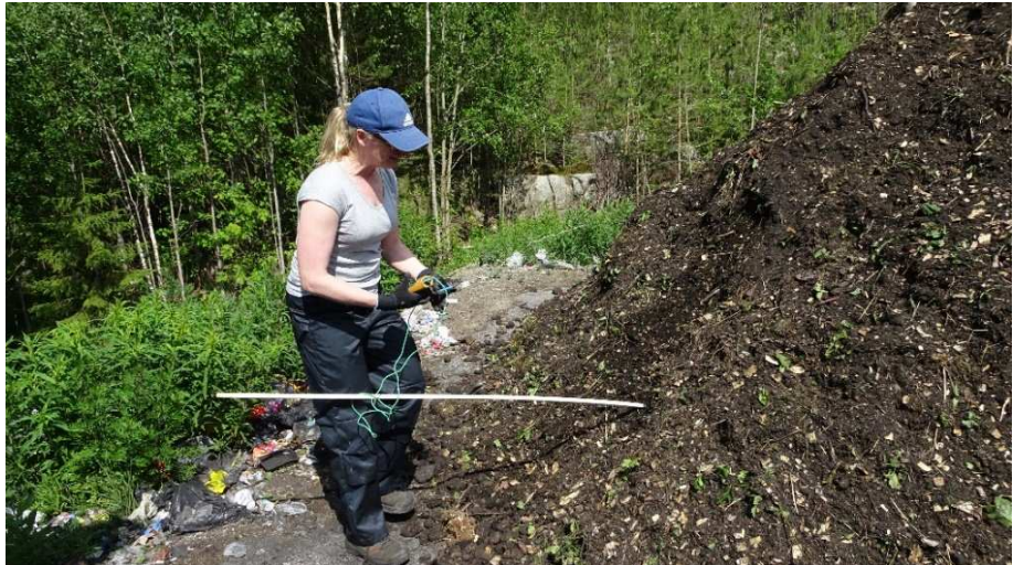
Figure 7. Measuring the temperatures of composting heaps.
