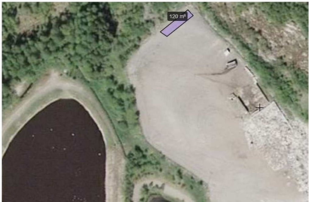
Figure 2. Pilot site at the waste treatment center. Waste waters are conducted to the settling tank and from there to municipal waste water treatment plant.
