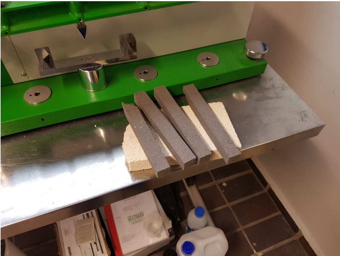
Fig. 5 Test bars and the bending strength test machine
