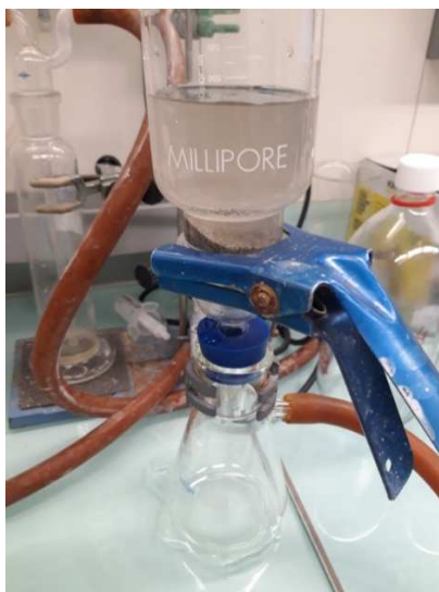
Figure 4: Filtering the sand
