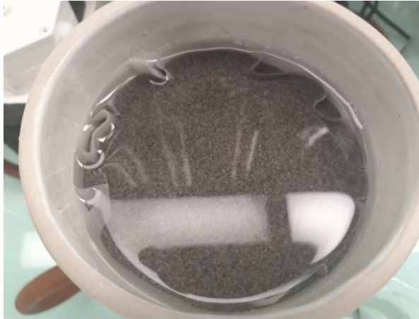
Figure 1: Washing sand with distilled water
