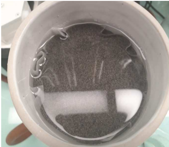
Figure 7: Washing sand with distilled water
