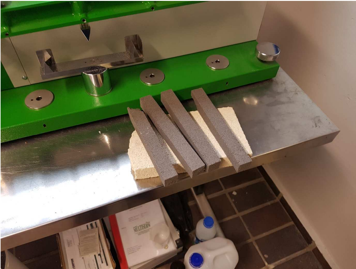
Fig. 17 Test bars and the bending strength test machine
