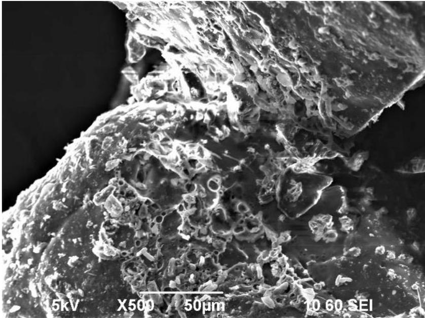
SEM photo of INOTEC sand to be treated: view of a chemical bridging and appearance of the residual gangue
