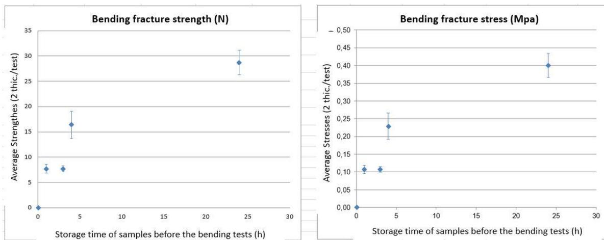
**With 100% of CTIF IE sand hydromechanically treated: bending fracture stress = 0.405 Mpa**
