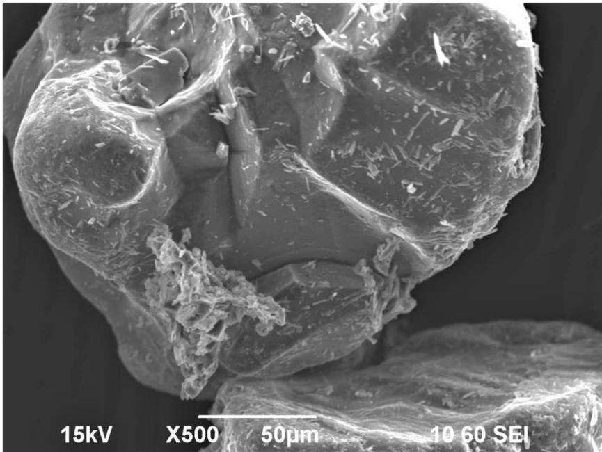
SEM photo of PEAK W37 sand to be treated: view of a chemical bridging and appearance of the residual gangue
