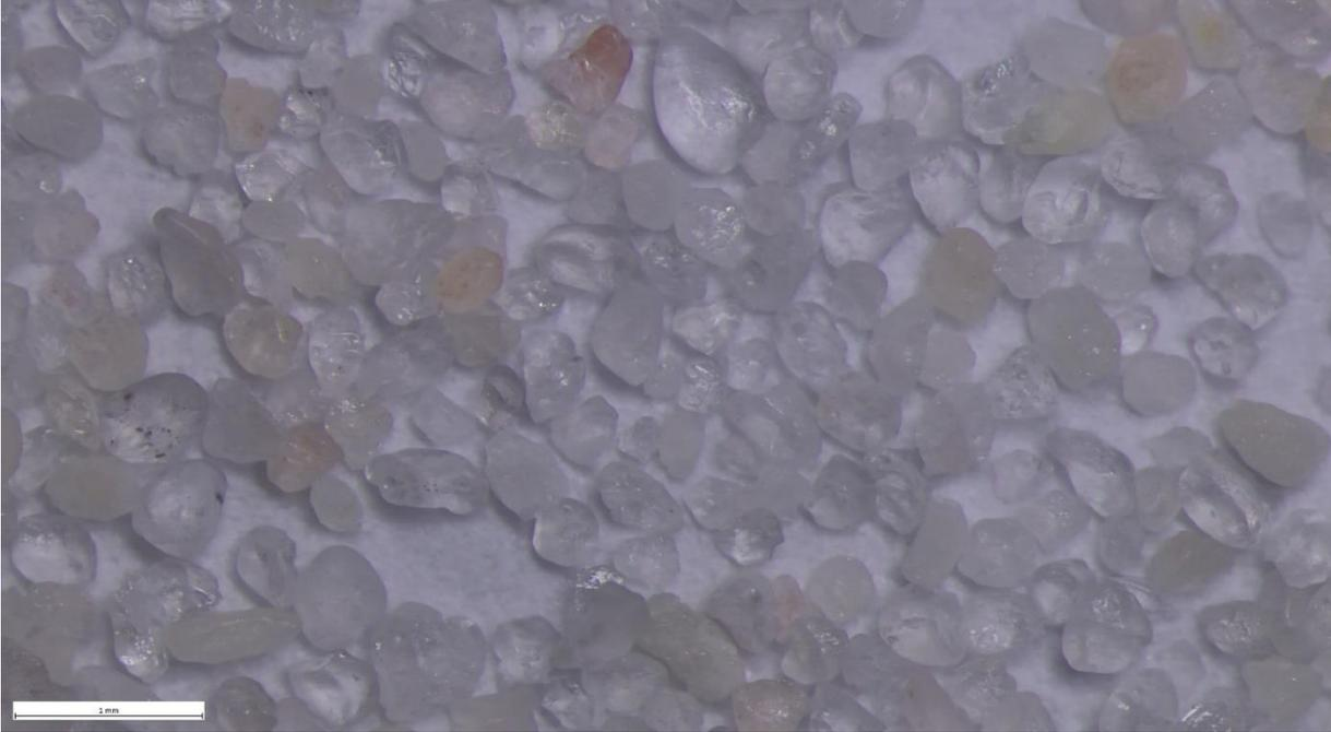
Photo - MEB new sand reference BE01: appearance of the grains
