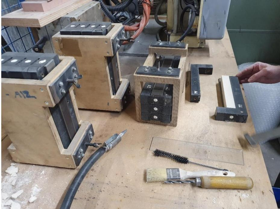
Measurement of flexural strength of test pieces
