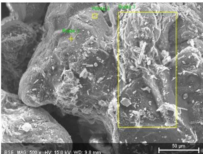
Photo of the sand to be treated marked GEOPOL W37-20, with the analysis zones " marked 1, marked 2, marked 3 ".
