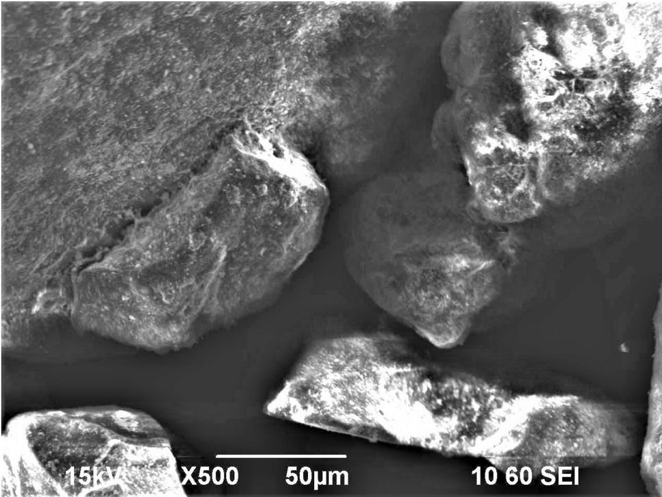
SEM photo of mechanically treated PEAK W37 sand: appearance of grains and residual gangue
