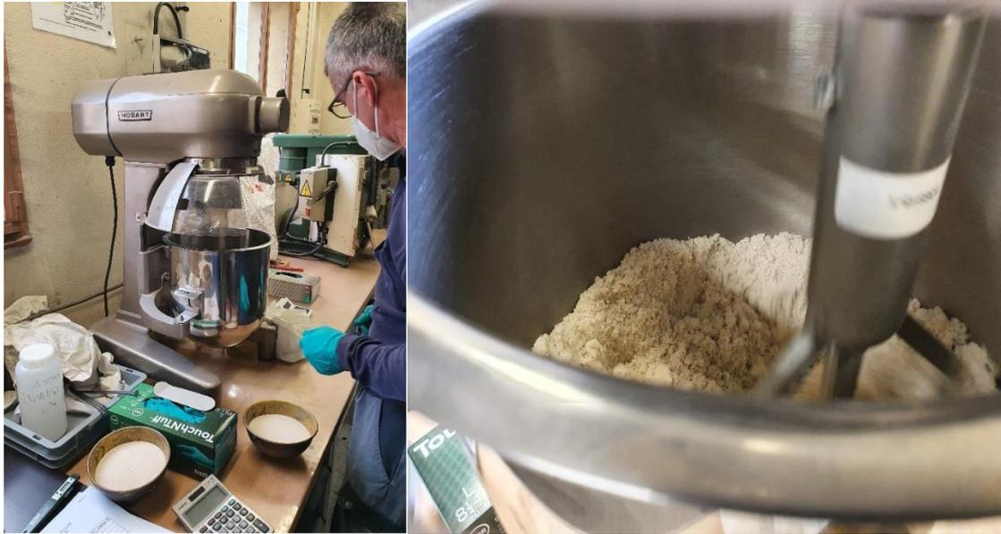
Equipment and tools used to produce cores (standardized test pieces)
