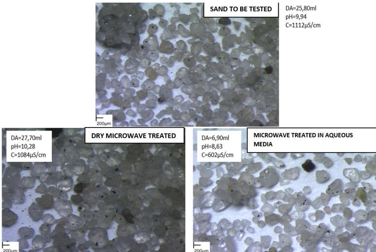
The treatment processes selected by CTIF for the Green Foundry Life project are those capable of cleaning inorganic sand waste to obtain a quality of treated sand sufficient for reuse in foundries (moulding, core making), or for external reuse.
