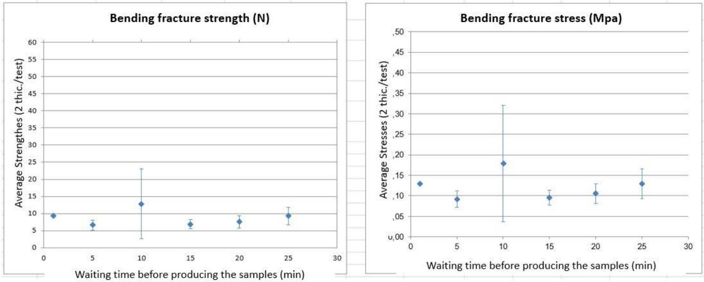
Comment: at T=30mn, hardening of the prepared sand and plugging of the machine's shooting head (unfilled test pieces)
