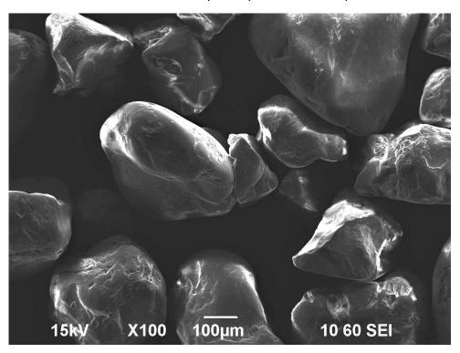
Photo MEB sand INOTEC treated by the hydromechanical process: overview
