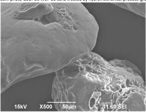
SEM photo of hydromechanically treated PEAK W37 sand: grain appearance
