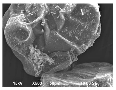
SEM photo of PEAK W37 sand to be treated: view of a chemical bridging and appearance of the residual gangue
