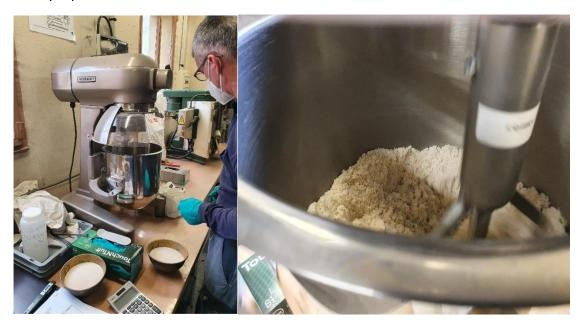
Equipment and tools used to produce cores (standardized test pieces)
