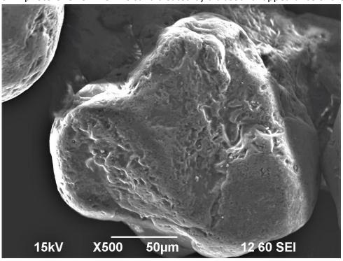
SEM photo of ultrasonically treated PEAK W37 sand: grain appearance
