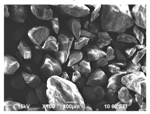
Photo MEB sand INOTEC mechanically treated: overview
