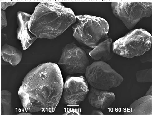
SEM photo of INOTEC ultrasonically treated sand: general view
