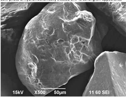
SEM photo of hydromechanically treated INOTEC sand: appearance of the grains
