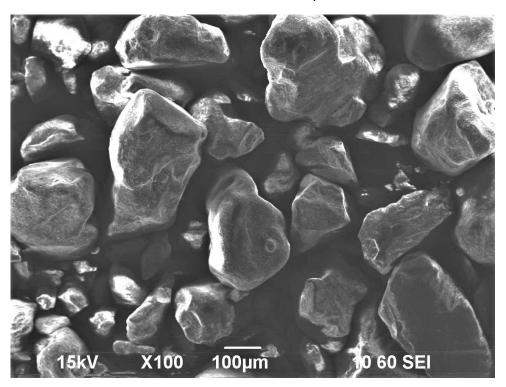
Photo MEB sand PEAK W37 mechanically treated: overview
