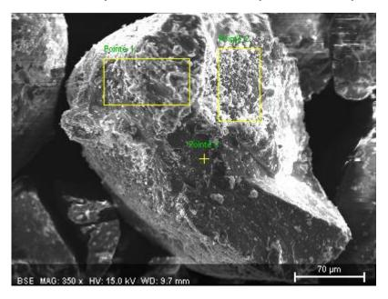
Photo of the sand to be treated, marked CTIF IE, with the analysis zones " marked 1, marked 2, marked 3 ".
