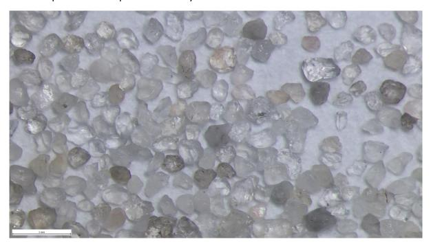
Photo - Optical microscope Ultrasonically treated PEAK W37 sand: overview
