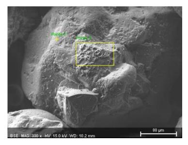
Photo of the sand to be treated marked PEAK W37, with the analysis zones " marked 4, marked 5 ".
