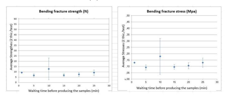
Comment: at T=30mn, hardening of the prepared sand and plugging of the machine's shooting head (unfilled test pieces)
