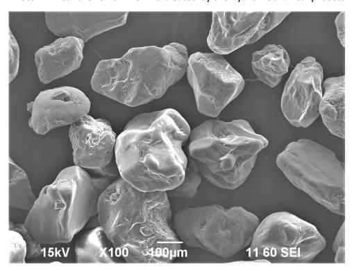
Photo MEB sand PEAK W37 treated by the hydromechanical process: overview
