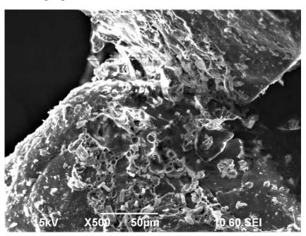
SEM photo of INOTEC sand to be treated: view of a chemical bridging and appearance of the residual gangue
