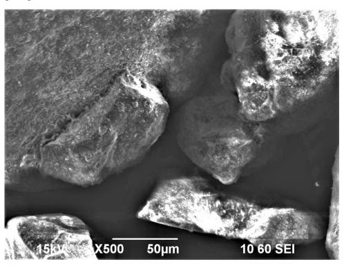
SEM photo of mechanically treated PEAK W37 sand: appearance of grains and residual gangue
