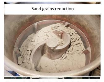
Homogenisation of the batch of sand to be treated
