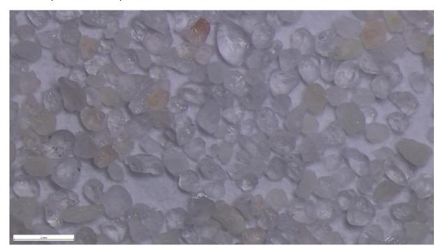
Photo - MEB new sand reference BE01: appearance of the grains
