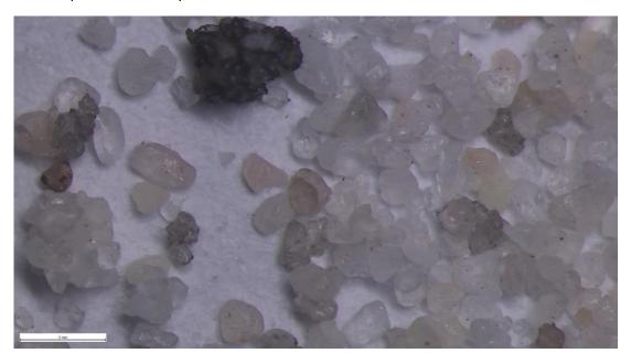
Photo optical microscope INOTEC sand to be treated: overview
