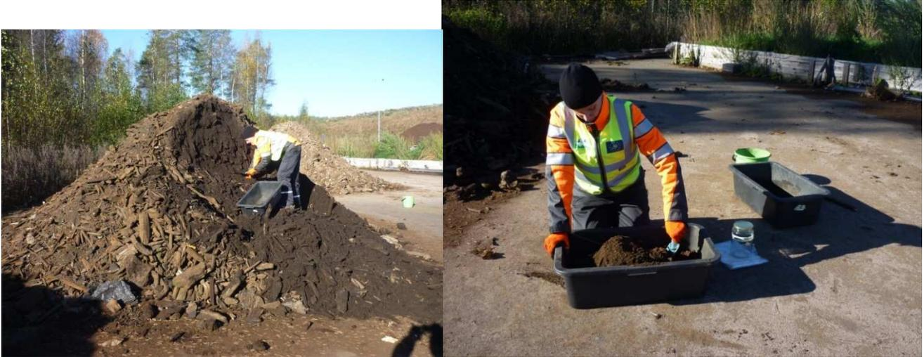
Figure 7. Composting material was analysed from each test heap in the beginning and in the end of each test period.
