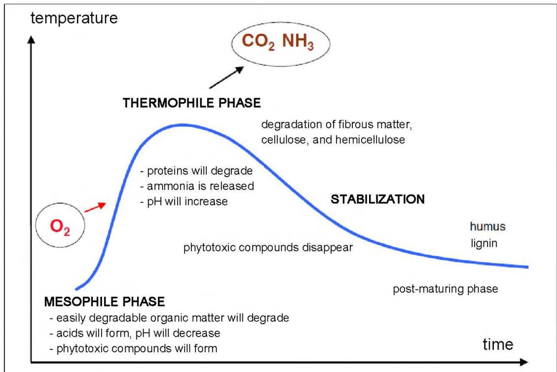
Figure 1. Different stages of the composting process (VTT 2006).
