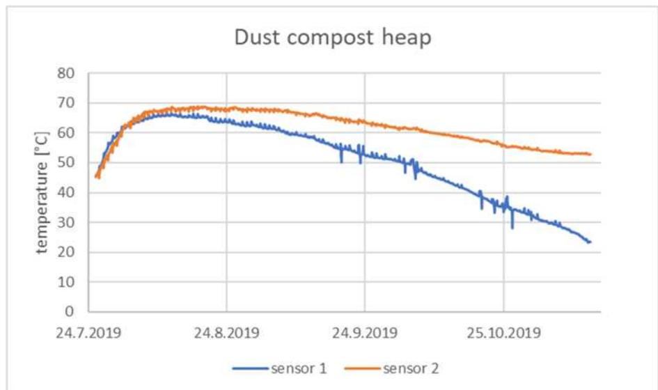
Figure 5. Temperature changes in dust compost test heap in two different depths in July-November 2019.
