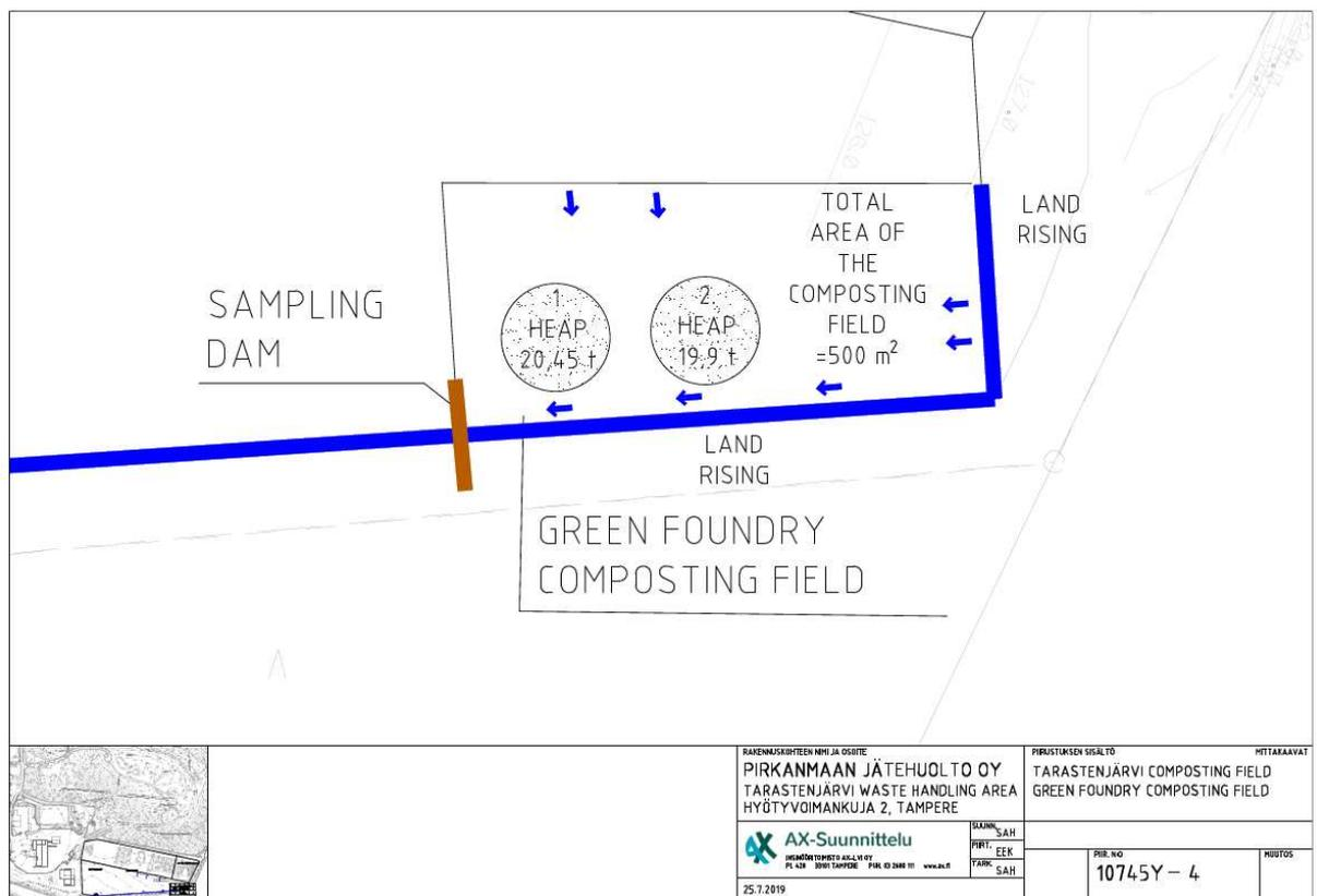
Figure 2. Composting test heaps at Tarastenjärvi in Tampere.
