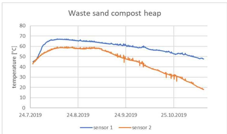
Figure 6. Temperature changes in waste sand compost test heap in two different depths in July-November 2019.
