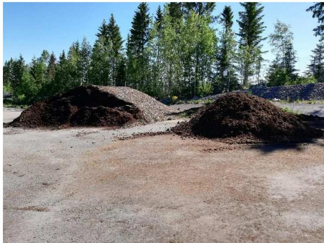
Figure 12. Constructing the composting test heap with inorganic binder system waste sand in June 2020.
