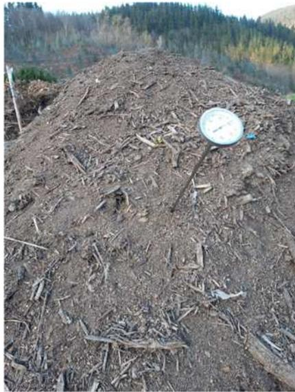
Figure 8: Manual thermometer used during sampling
