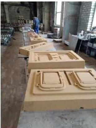
Photo 54. Test moulds after stripping
