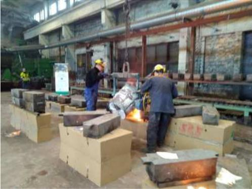
Figure 63. Example of pouring into tested Geopol moulds. Small leakage in one mould, left.
