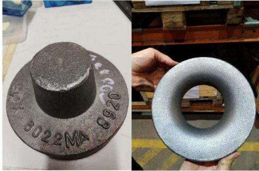
Photo 46. Surface qualities of castings made by inorganic binder nr.3 (left) and Alphaset (right).
