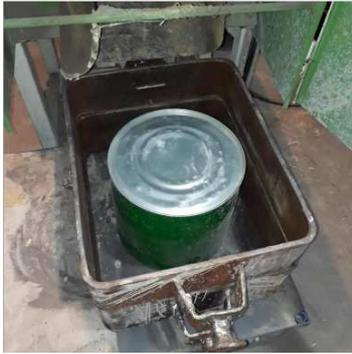
Photo 3. Steel barrel as a pattern.
