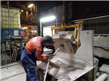
Photo 42. Coating of the test moulds
