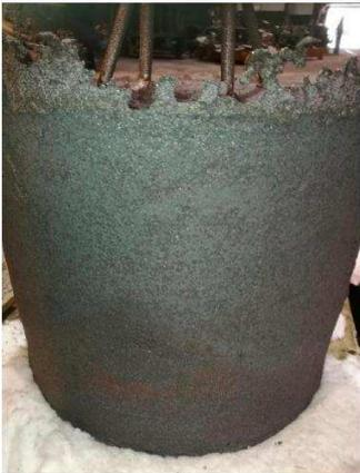
Photo 10. Surface quality of the chamber test cast.
