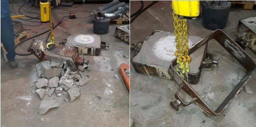
Photo 9. Breaking of the chamber test mould.
