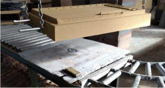
Photo 60. Mould made by Geopol, broken during stripping
