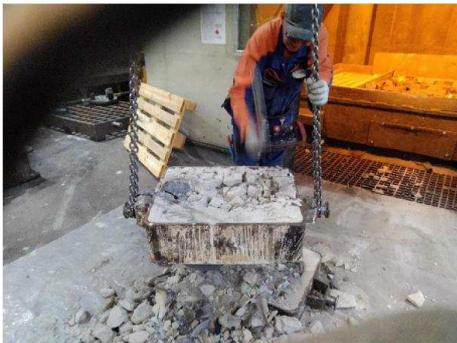
Photo 45. Manual crushing of moulds
