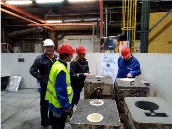
Photo 16. Part of the test moulds on a casting wagon.
