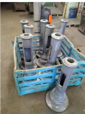
Figure 65. Test casting made by Geopol binder system.
