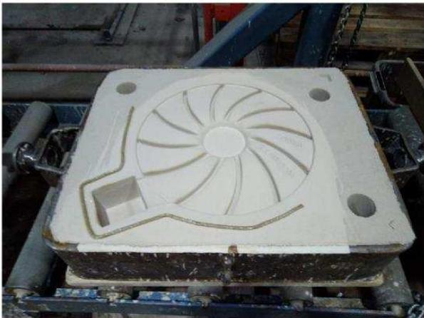
Photo 22. An example of coated mould.
