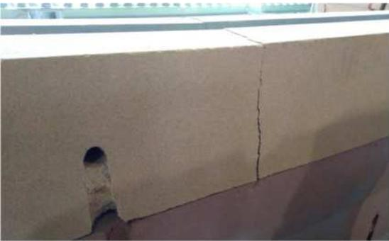
Photo 61. Mould made by Geopol, broken after stripping
