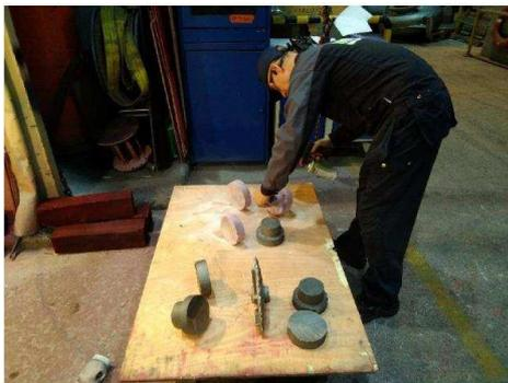
Photo 28. Dye penetrant inspection (DPI)
