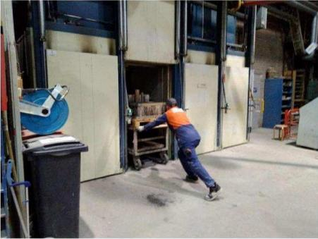
Photo 14. Core heating furnace.
