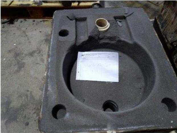
Photo 18. Cracks in the test mould due the high strength.
