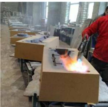
Photo 62. Drying of the coating of Geopol moulds with flame burning.
