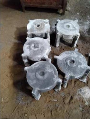
Photo 58. Test castings before shot blasting.
