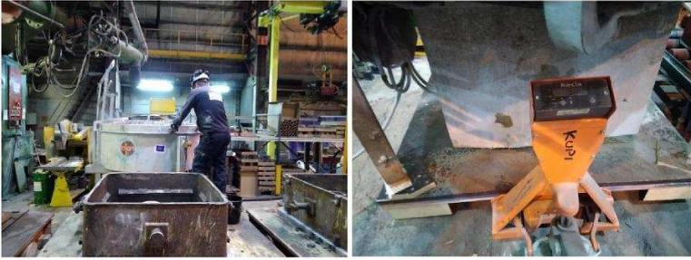
Photo 11. The mixer and the method for measuring the amount of sand
