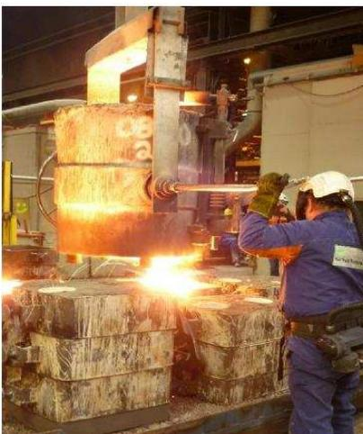
Photo 17. Pouring of melted metal into the inorganic test moulds.
