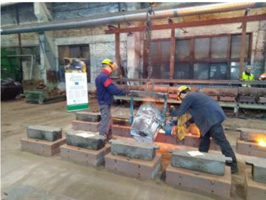
Photo 56. Pouring into test moulds made by Peak's binder system
