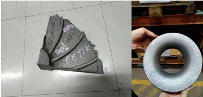
Photo 27. Surface quality of castings made by using inorg. binder nr.2 (left) and Alphasert (right)
