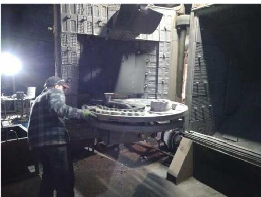
Photo 57. Shot blasting machine in Valumehaanika.
