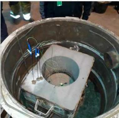
Photo 5. Test mould in the chamber, thermocouples installed.
