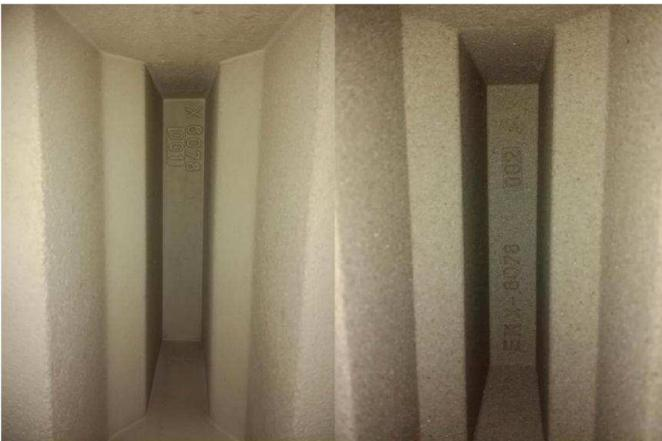
Photo 19. Coated mould, left and uncoated mould, right.
