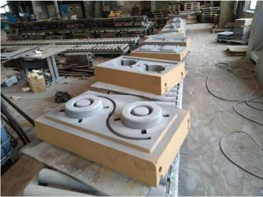
Photo 55. Coated test moulds made by Peak's binder system
