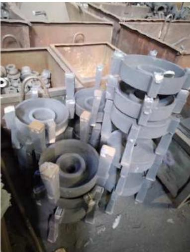
Photo 59. Photo 58. Test castings after shot blasting.
