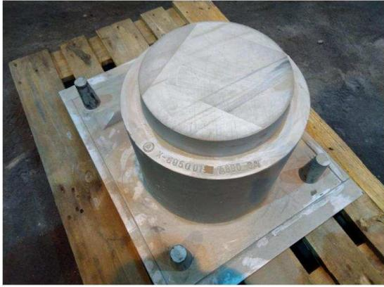
Photo 32. The pattern for the chamber test mould
