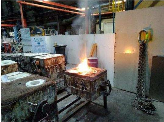
Photo 44. Fumes from an Alphasbet mould
