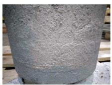
Photo 38. Surface quality of the chamber test casting (after sand blasting), no coating was applied.
