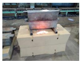
Photo 64. Geopol test mould. No visible fumes were emitted (5 min after pouring).
