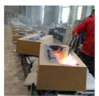
Photo 62. Drying of the coating of Geopol moulds with flame burning.
