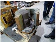
Photo 15. Breaking of a core, due to lack of proper drying
