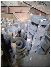
Photo 59. Photo 58. Test castings after shot blasting.
