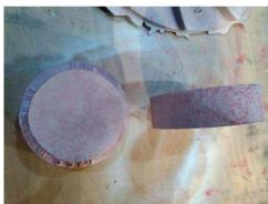
Photo 29. Dye penetrant inspected test castings. No cracks or gas porosity holes existed.
