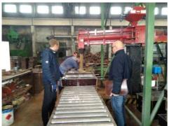
Photo 53. Hand moulding in Valumehaanika
