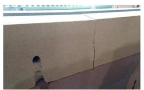
Photo 61. Mould made by Geopol, broken after stripping
