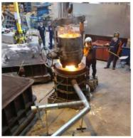
Photo 7. Chamber test casting.
