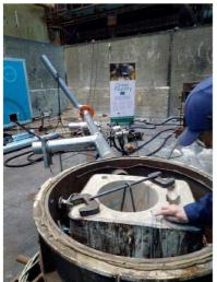
Photo 34. Test mould inside the chamber. The locations of the thermoelements.
