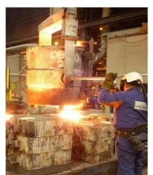
Photo 17. Pouring of melted metal into the inorganic test moulds.
