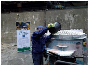
Photo 30. Test mixer, adding of binder during mixing
