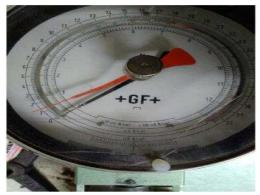
Photo 41. The result of sand bar bending test after 24 h.
