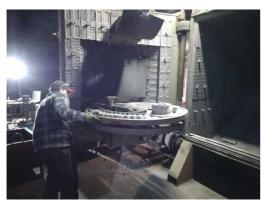
Photo 57. Shot blasting machine in Valumehaanika.
