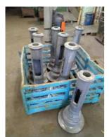
Figure 65. Test casting made by Geopol binder system.
