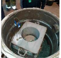
Photo 5. Test mould in the chamber, thermocouples installed.
