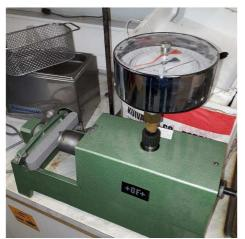
Photo 2. Bending strength test machine.
