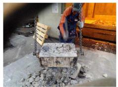
Photo 45. Manual crushing of moulds
