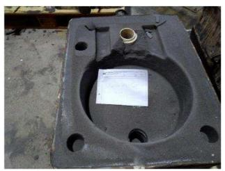
Photo 18. Cracks in the test mould due the high strength.
