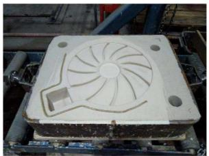
Photo 22. An example of coated mould.
