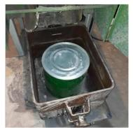
Photo 3. Steel barrel as a pattern.
