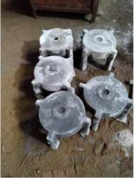
Photo 58. Test castings before shot blasting.
