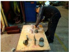
Photo 28. Dye penetrant inspection (DPI)
