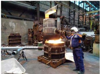
Photo 35. Pouring into the chamber test mould
