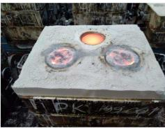
Photo 24. No fumes from the mould
