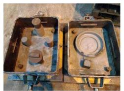
Photo 40. The patterns of one test mould
