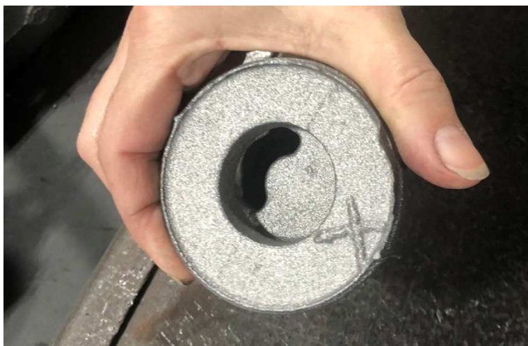
Figure 38 Casting after shot blasting process – Type X
