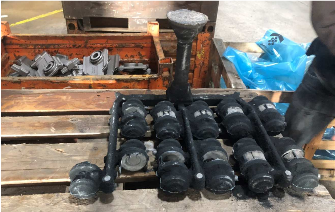
Figure 31 Castings before the knocking
