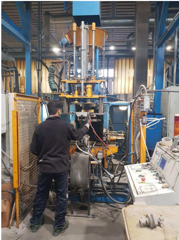
Figure 5 Excess sand removal
