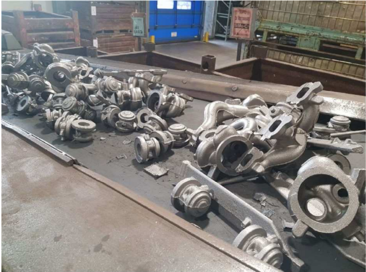
Figure 36 External shot blasting process on carpet blasting machine
