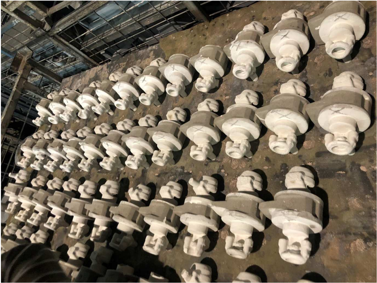
Figure 26 Cores before the insertion into the mould
