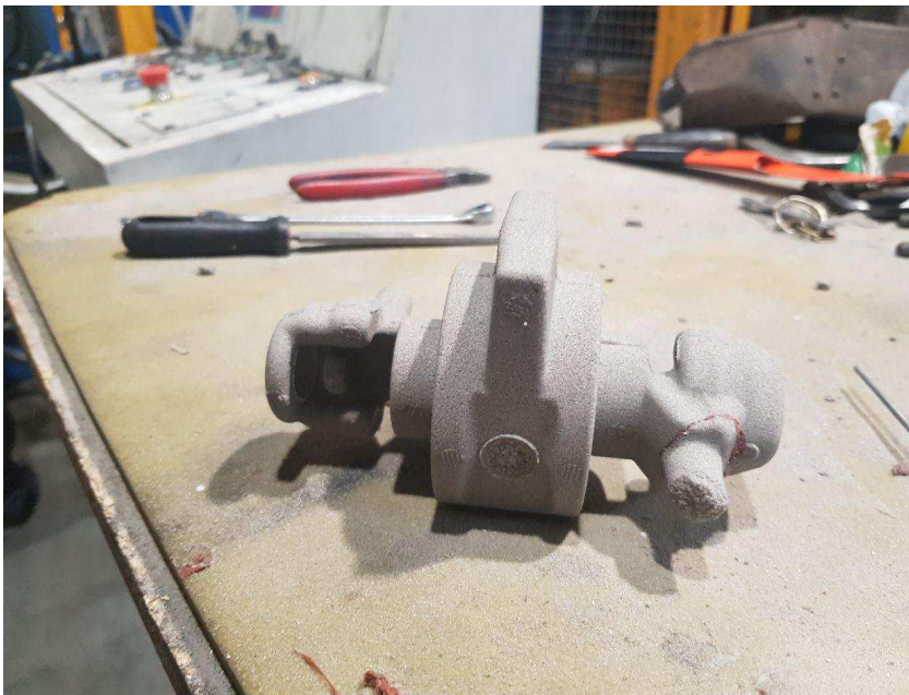
Figure 7 Inorganic core with surface break
