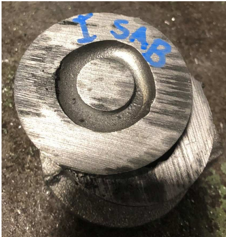
Figure 41 Casting Type I after cutting operation
