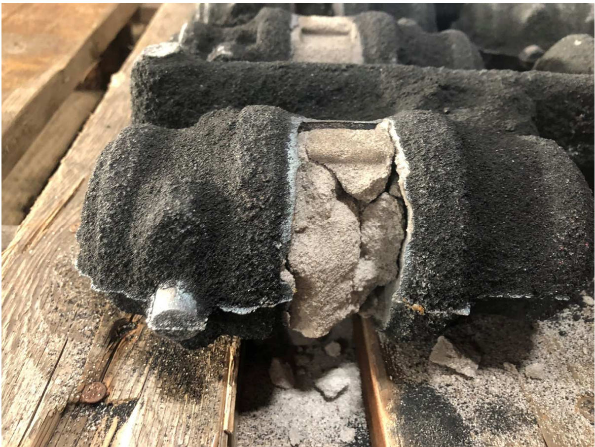
Figure 32 Detail of one casting before the knocking
