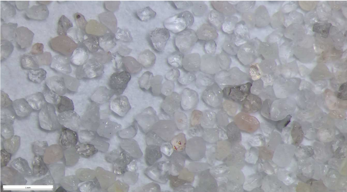
Photo - optical microscope ultrasonically treated CTIF IE sand: overview
