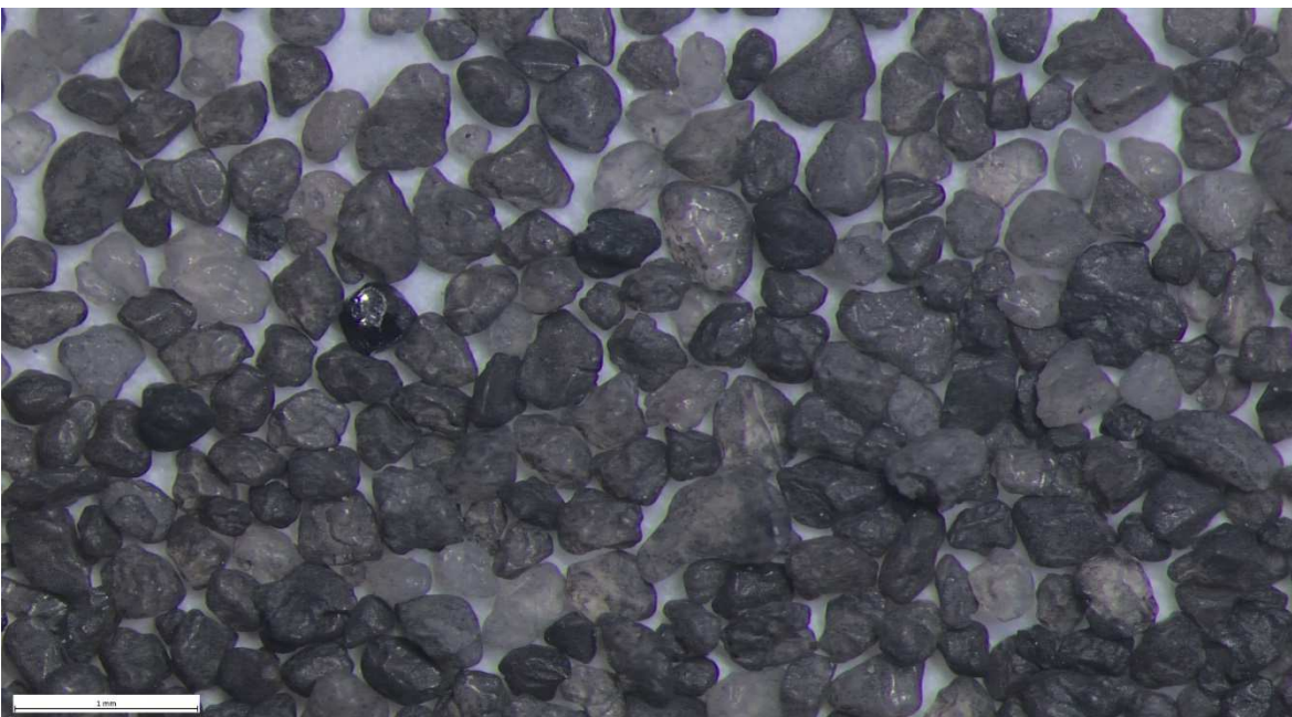
Photo - optical microscope sand INOTEC mechanically treated: overview
