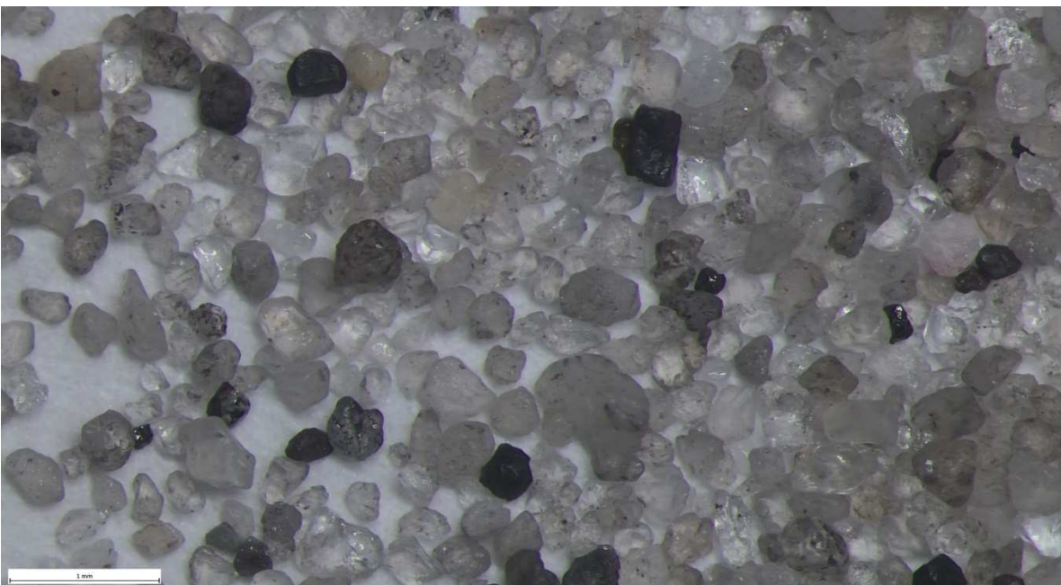
Photo - Optical microscope Ultrasonically treated INOTEC sand: overview
