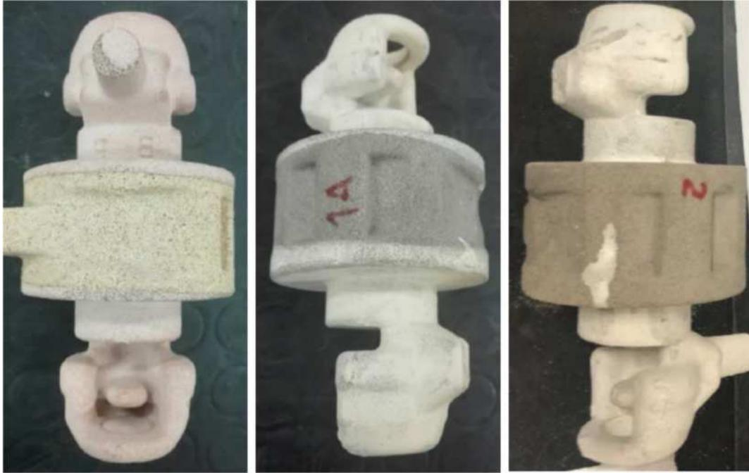
Figure 2: Comparison of the three different types of cores (left to right, organic binder, inorganic binders 2 and 3).
