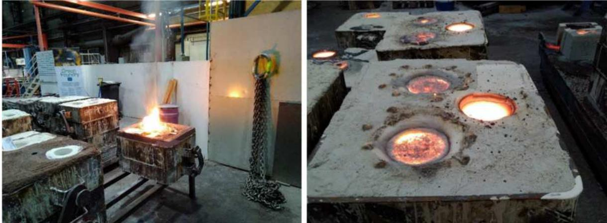
Figure 1: Emission from an Alphaset-bonded mould (left) and another one based on a hybrid binder (right, binder 5). Images were taken approx. 4 minutes after pouring in both cases.
