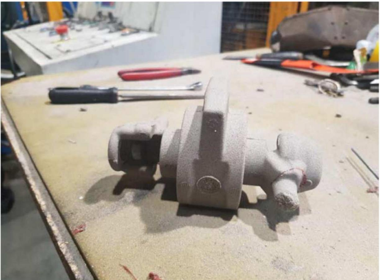
*Figure 3: Example of a core with visible surface defects.*
