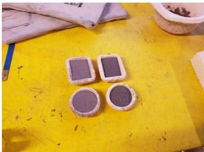
Fig 29. Loss on Ignition samples
