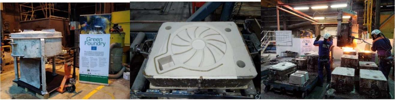
Figures 6-8. Castings with three different inorganic binders were produced at Karhula foundry.
