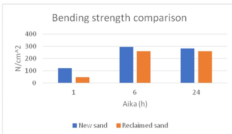
Fig. 34 Bending strength results for Furan bonded sand
