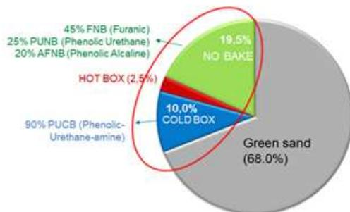
Figure 1: All foundry moulding systems, including green sand. Source: Courtesy of Huttenes Albertus Ilarduya
