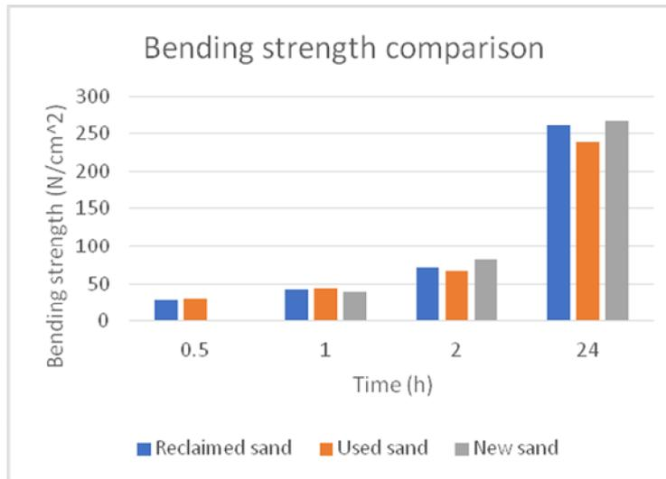
*Fig. 31 Peak bending strength results*
