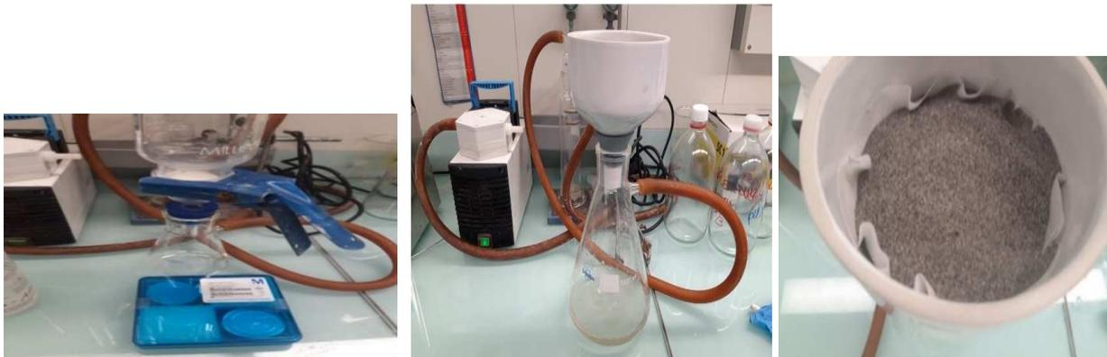
Fig 22-24. Büchner funnels equipment and filtering the sand after washing.
