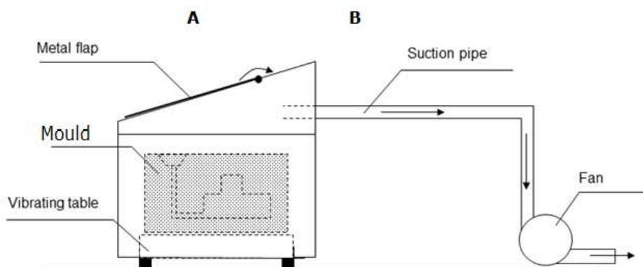
Figure 39. Test arrangements in Hardkop iron foundry.
