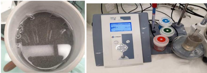
Fig 20-21. Washing sand with distilled water and pH measurement
