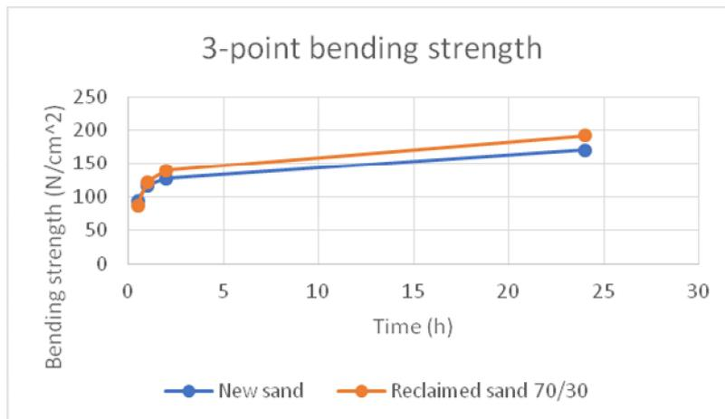
Fig. 33 Bending strength results for APNB sands
