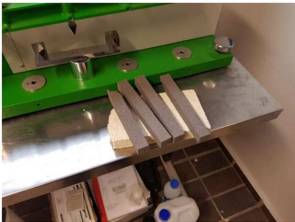
*Fig. 30 Test bars and the bending strength test machine*
