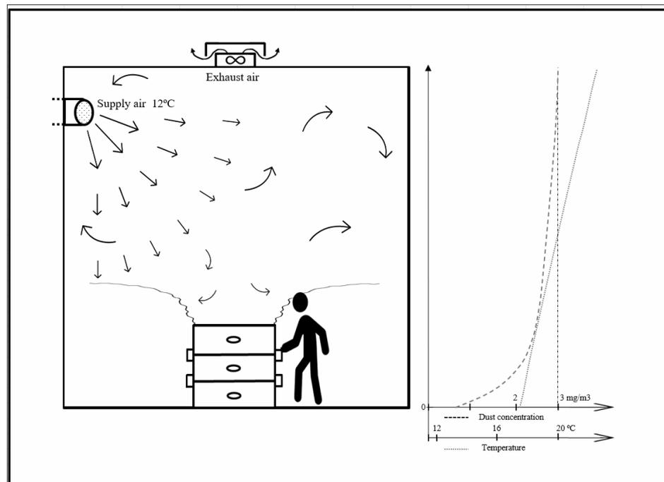
Fig 41. In case of displacement ventilation  $k_2 \approx 1,0$  (mixing ventilation).
