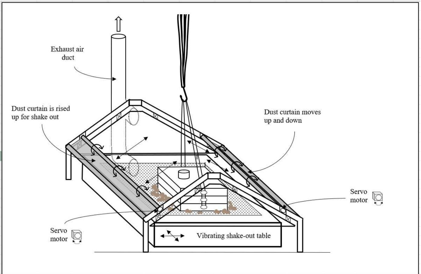
Fig 43. Local exhaust system of the shake-out.
