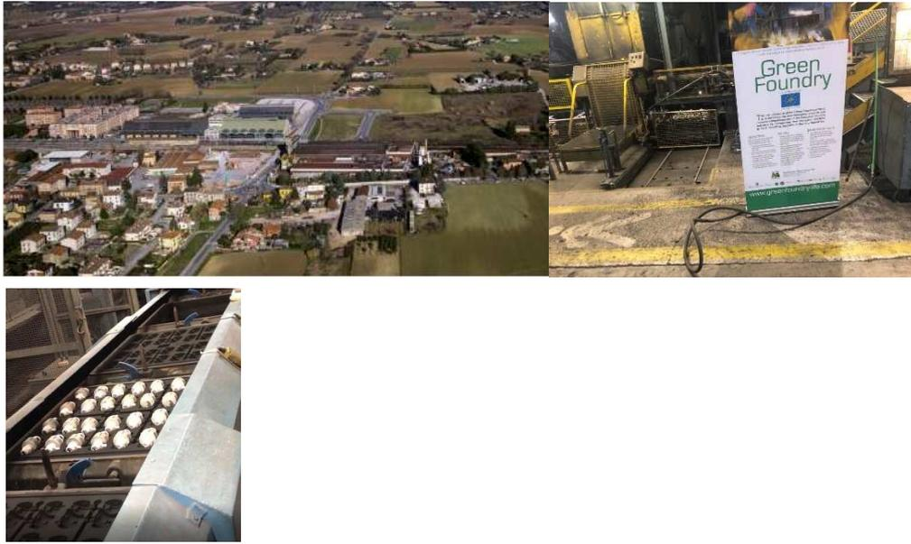
Figures 3-5. Cores with inorganic binders were produced at FOM Tacconi foundry.
