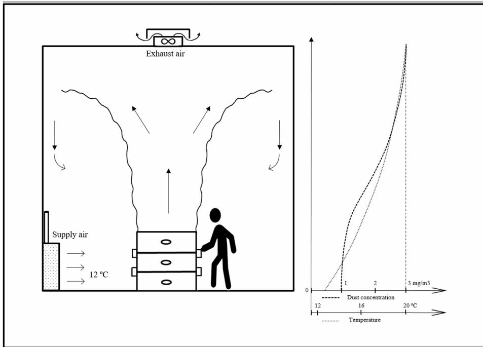
Fig. 40. In case of displacement ventilation  $k_2 \approx 0,3$ .
