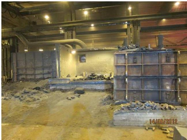
Fig 44. Shake-out with local ventilation but without any enclosure.
