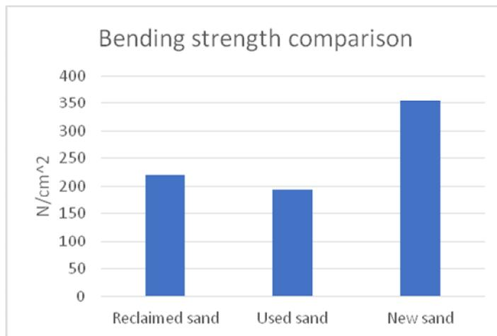
Fig. 32 Bending strength results of Inotec
