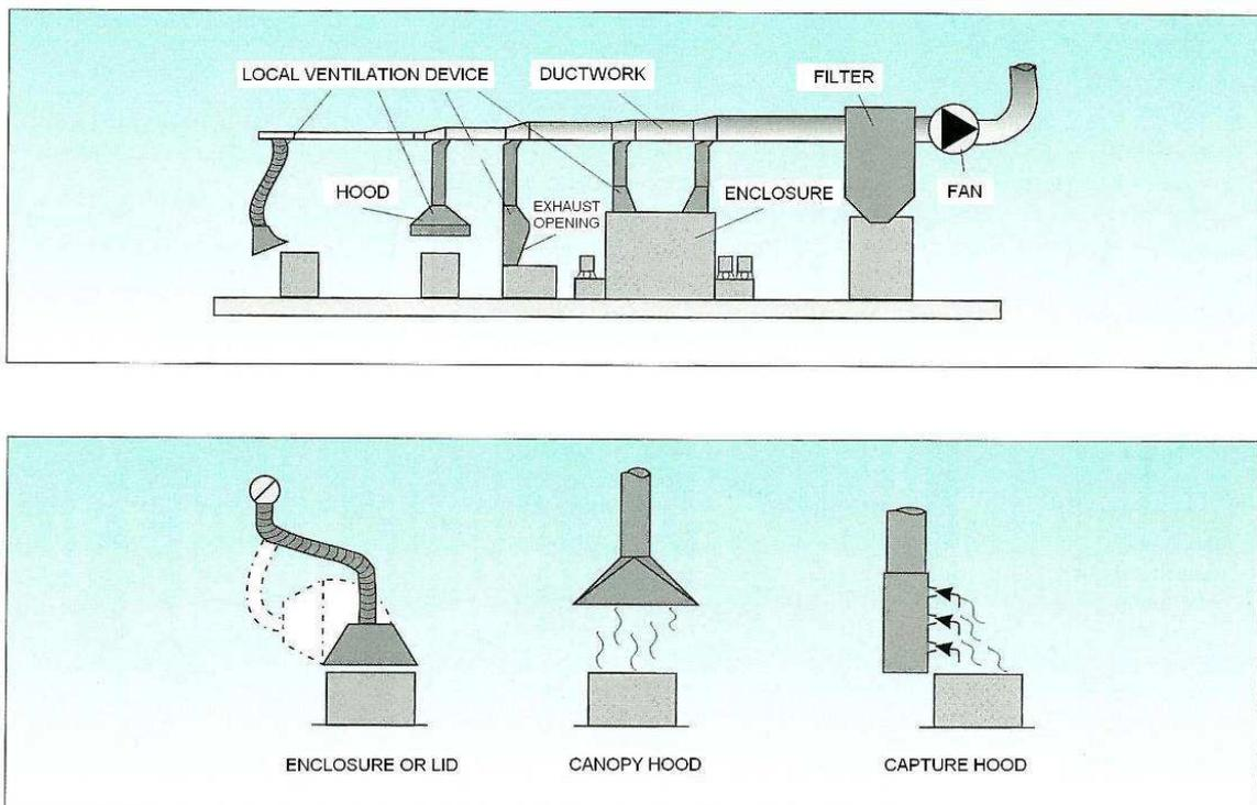
Figure 42: Local ventilation efficiency is the capture efficiency of contaminants from the emission source.
