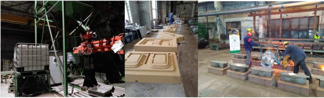
*Figures 9-11. Test casts with two different inorganic binders were produced at Valumehaanika foundry.*
