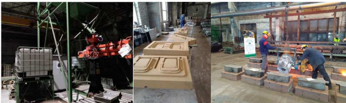
Fig. 5. Test casts with two different inorganic binders were produced at Valumehaanika foundry.
