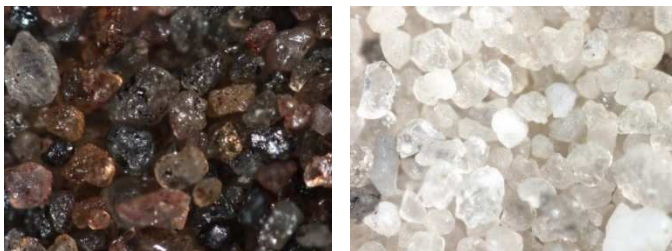
Figure 9. Stereomicroscopy photos of unreclaimed vs. reclaimed APNB sand.
