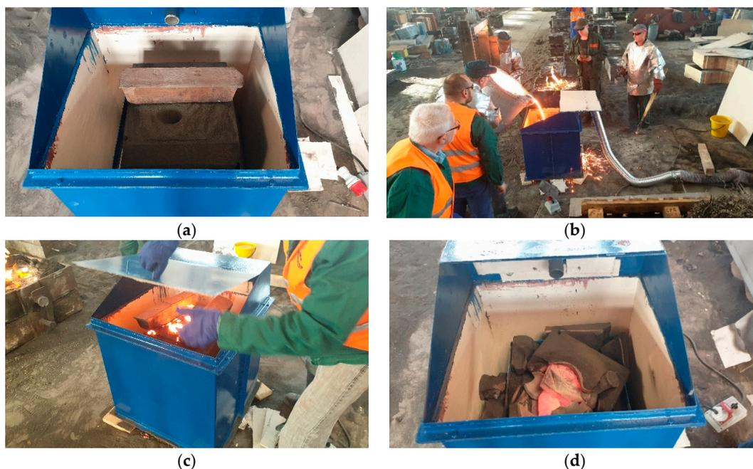
**Figure 2.** The view of the testing unit during different stages of the tests (a) mould sand prepared for pouring (b) pouring the mould sand (c) cooling of the mould sand (d) knocking out the casting.
