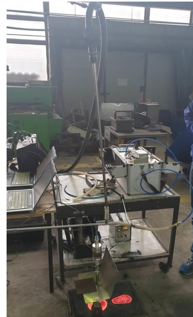
Scheme of the stand for measuring of the gas volume and BTEX and PAHs emission.
